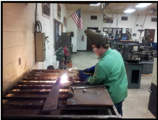
PHS student Jacob White uses a cutting torch to cut a piece of metal for practicing shielded metal arc welding.
